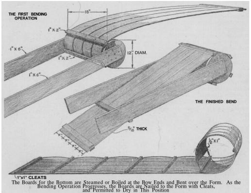
two others. Nail the end of one of the 6-ft. boards to each end of the block, so that their extended ends are parallel.
