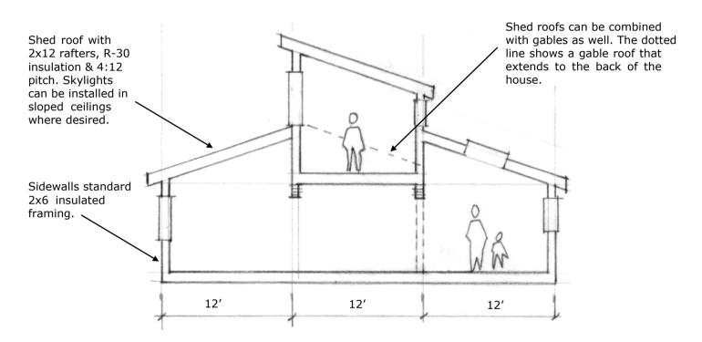
Three structural bays of 12' width. The second floor loft joists are carried by a combination of bearing walls and beams. Foundation support is needed below. These three sections need not be built all at one time. The dotted wall could have been opened up when the right hand bay was built later than left hand two bays.
