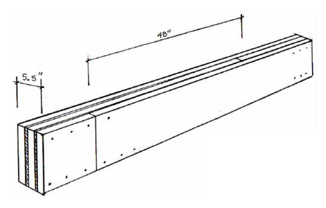
While this is not an engineered beam and may not be approved by all inspectors, a careful builder can construct a strong and durable beam of almost any length from 2x joist lumber, plywood and construction adhesive. A three joist beam with 2x12's and two layers of 1/2" plywood as shown above will have roughly the same strength as a 6x12 beam of the same lumber and grade. It will also be the same width and can therefor use the same hardware such as post brackets, hangers and post caps.
