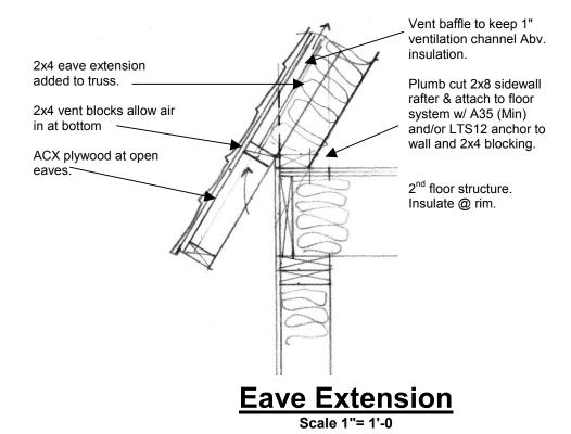
Adjust this structural configuration so it is appropriate for your spans and local wind, snow and earthquake loads. Consult your local building department or a structural engineer.
